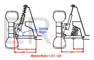
So the equation for Wheel Rate is the Motion Ratio squared times the Spring Rate.
